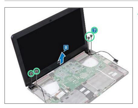
Replace the four screws (M2x5) that secure the display assembly to the computer base.
