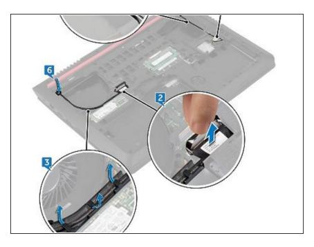
Slide the display cable and antenna cables through the slots on the computer base.
