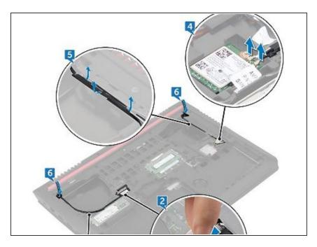
Connect the display cable to the system board.
