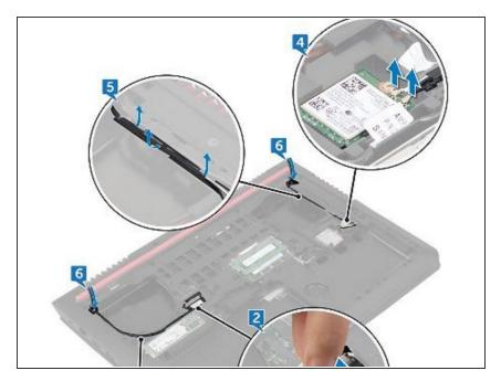
Note the antenna-cable routing and remove the antenna cables from the routing guides on the computer base.
