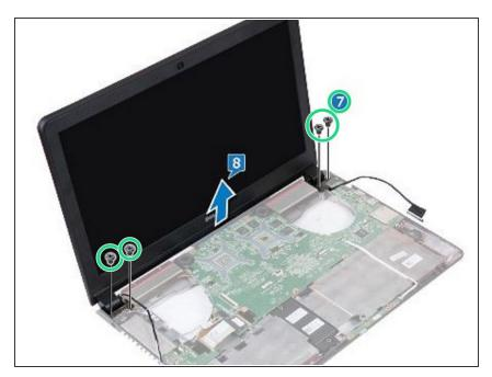
Remove the four screws (M2x5) that secure the display assembly to the computer base.
