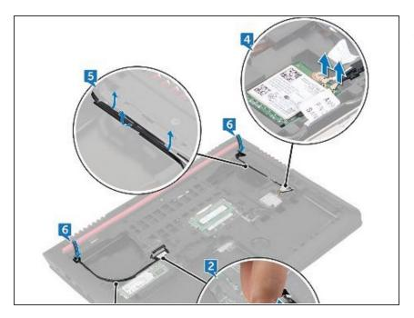
Slide the display cable and antenna cables through the slot on the computer base.
