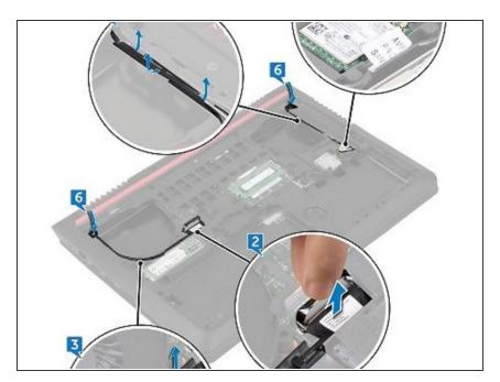
Note the display-cable routing and remove the cable from the routing guides on the computer base.
