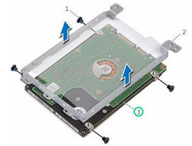
Lift the hard-drive bracket out of the hard drive.
