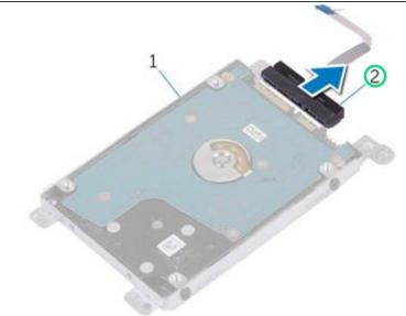
Disconnect the interposer from the hard-drive assembly.
