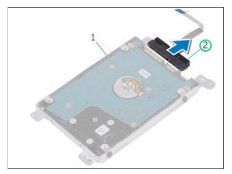
Connect the interposer to the harddrive assembly.
