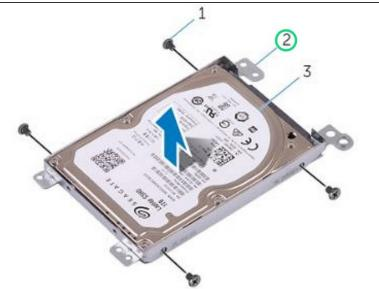
Lift the hard drive off the hard-drive bracket.
