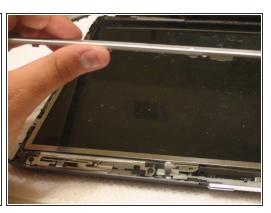
Mhen removing the bezel be careful not to damage it. Removal should be done gently and slowly.
