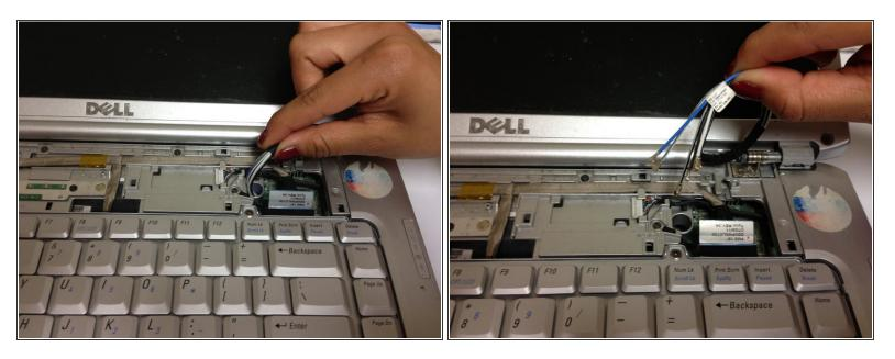
Pull the wires that you disconnected in the previous step through the hole in the top of the laptop.
