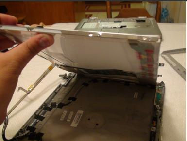
Carefully lift and remove the LCD display with both hands.
