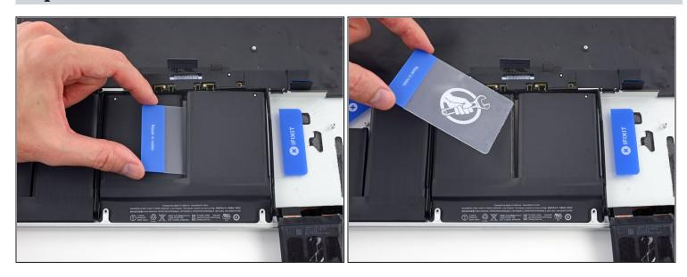
• Remove the first plastic card that you inserted under the center-right battery cell.
