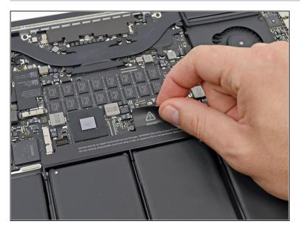
Peel back the warning label covering the battery connector.
