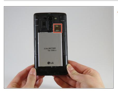
Using your fingers or a plastic opening tool, eject the micro SD card from the device.
