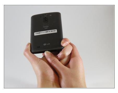
Using your fingers or a plastic opening tool, remove the back cover from the device.
