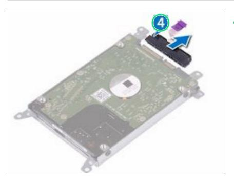
Disconnect the interposer from the hard-drive assembly.
