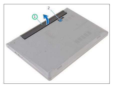
Lift the battery at an angle and remove the battery from the battery bay.
