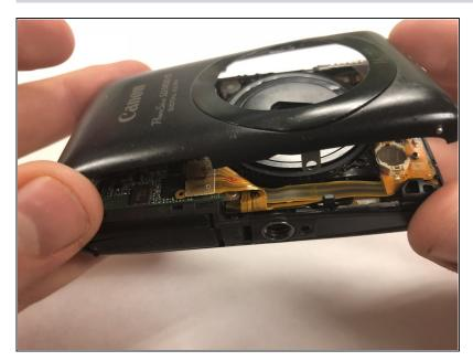
• Remove the front face panel off of the camera.
