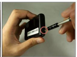
• Remove the four 2mm Phillips #00 screws on both sides of the camera.
