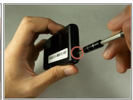
Remove two 2mm Phillips #00 screws on both sides of the camera.
