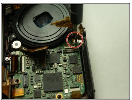
Remove the three 3mm Phillips #000 screws from the motherboard.
