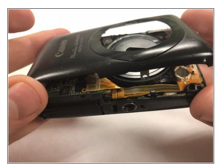
Remove the front face panel of the camera.
