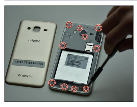
Remove all ten 0.4 mm screws with a Phillips #00 screw bit.
