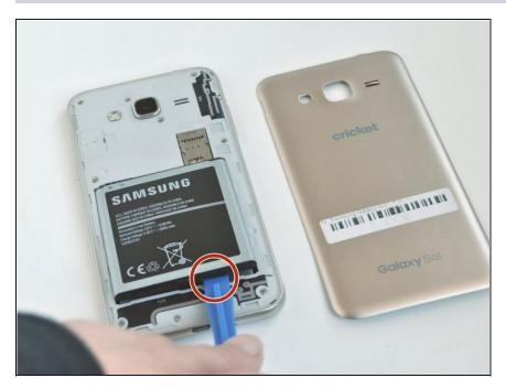
Remove the battery by lifting from the bottom up with an opening tool or a small flat tool such as a credit card.
