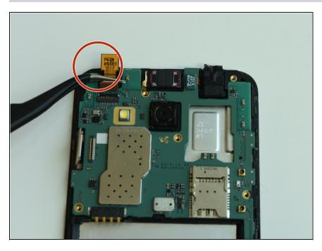
Remove the front camera at the top left of the phone be carefully removing it with tweezers.
