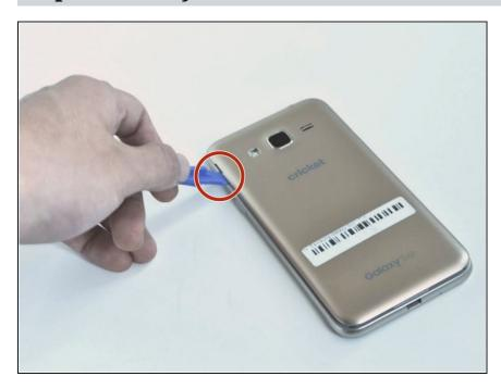
Remove the back case of the phone by using an opening tool or fingernail to lift the divot on the top left side.
