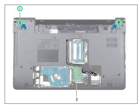
Turn the computer over and replace the two screws that secure the display assembly to the computer base.
