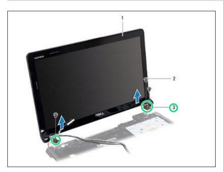
Use the alignment posts to place the display assembly on the computer base.
