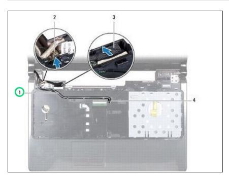
Note the routing of the Mini-Card antenna cables and remove them from the routing guides on the palm rest.
