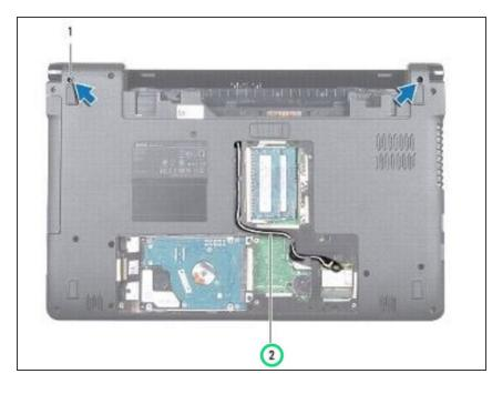
Route the Mini-Card antenna cables through the routing guides on the palm rest.
