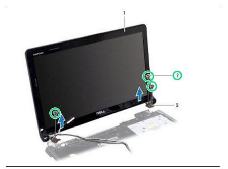
Replace the three screws that secure the display assembly to the computer base
