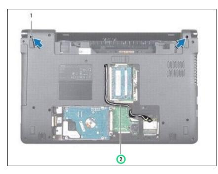
Thread the Mini-Card antenna cables through the slot in the computer base.
