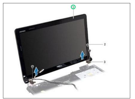
Lift the display assembly off the alignment posts on the computer base.
