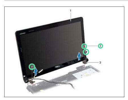
Hold the display assembly in place and remove the three screws that secure the display assembly to the computer base.
