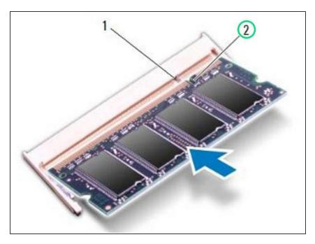
Align the notch on the **NEW** memory module with the tab in the memorymodule connector.
