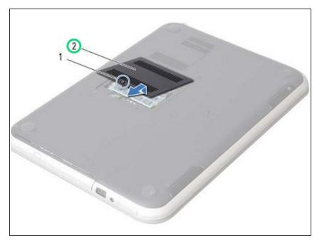
Using your fingertips, lift and slide the memory-module cover out of the slots on the computer base.
