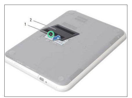
Loosen the captive screw that secures the memory-module cover to the computer base.
