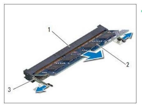
Align the notch on the NEW memory module with the tab on the memorymodule connector.
