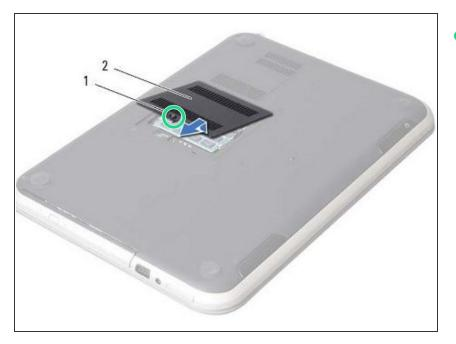
Tighten the captive screw that secures the memory-module cover to the computer base.
