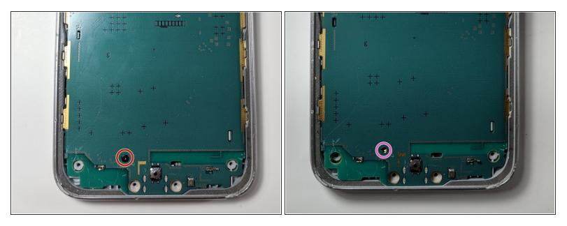
• Remove the one black screw located below the bottom plastic piece.
