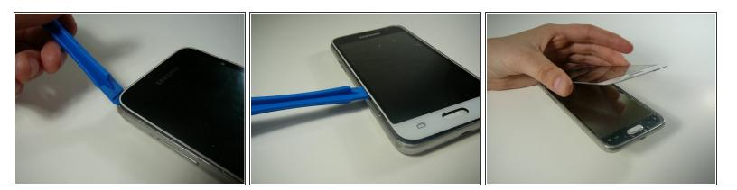
Use a Thin Plastic Tool (such as a guitar pick) or Plastic Prying Tool (such as a spudger) to lift out the glass digitizer and LCD screen around the edges.
