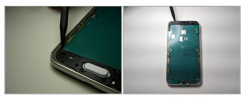
• Using a spudger to remove the black plastic pieces on the top and bottom of the screen.
