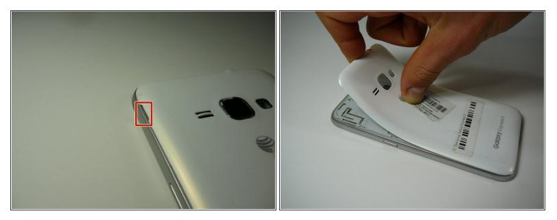
Locate the indent area highlighted in red and use either your fingernail or a Prying Tool (such as a guitar pick) to separate the back from the body of the phone.
