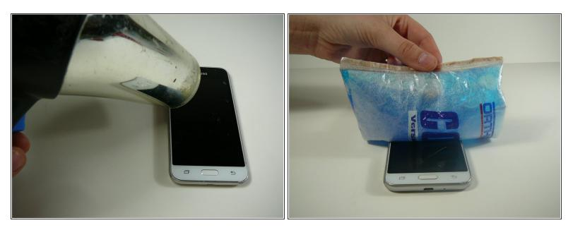
• Use a blow dryer or heating pad to heat up the screen.
