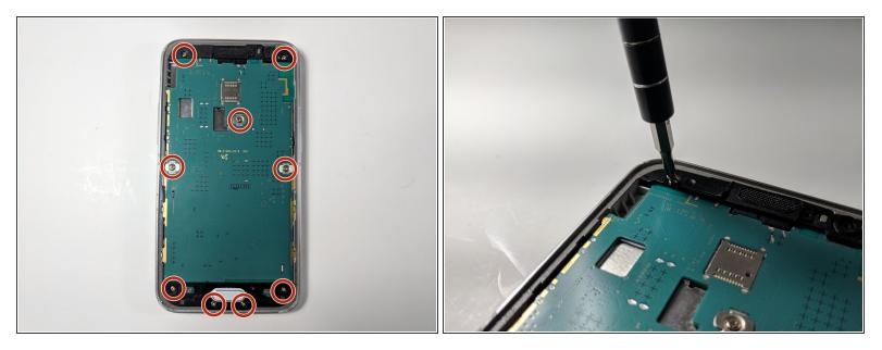
• Remove the nine screws with a Phillips #0 screwdriver.
