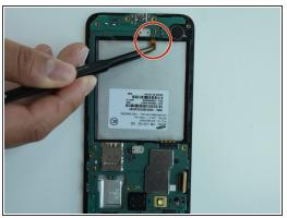
After removing the grey part of the phone, you will need to remove the motherboard by detaching all the chips.
