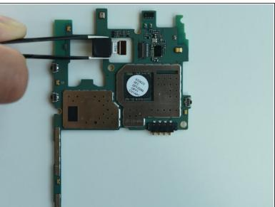
To remove the rear camera, flip the tab upward and then pull the camera straight out.
