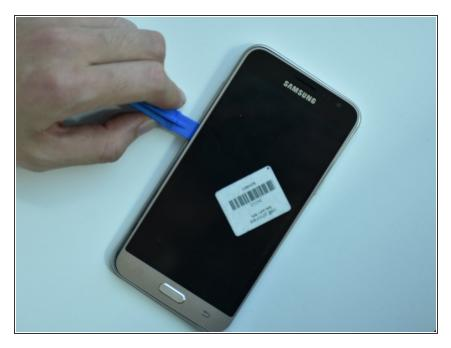
After you have removed all the screws, take a credit card or plastic tool to lift the screen. You will go all around the border of the phone.
