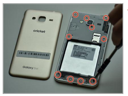
Remove all ten 0.4mm screws by unscrewing them with the Phillips #00 screwdriver. After this, you will be able to lift up and remove the grey plastic piece.
