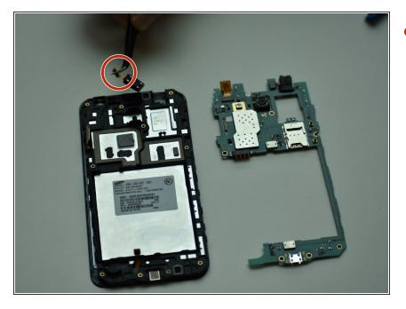
Using the curved tweezers, grab ahold of the gold piece of the speakers and slowly lift out of the speaker slot.
