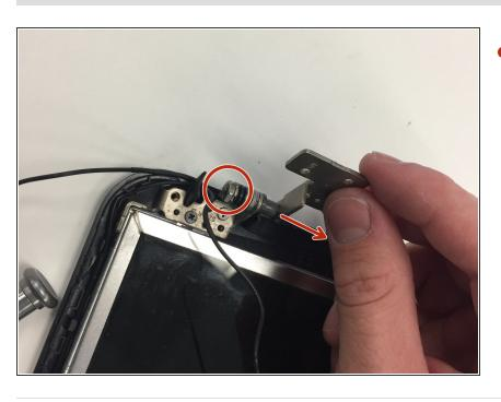
Use a pair of pliers to unscrew the nut and pull out the hinge.
