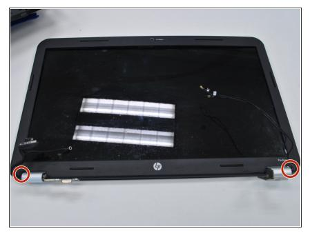
Remove the sticky tabs on the bottom of the screen just outside the hinges, and remove the two screws underneath.
