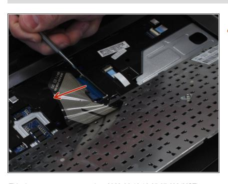
Flip up the black tab holding the keyboard in place via the ribbon cable and pull out the cable
