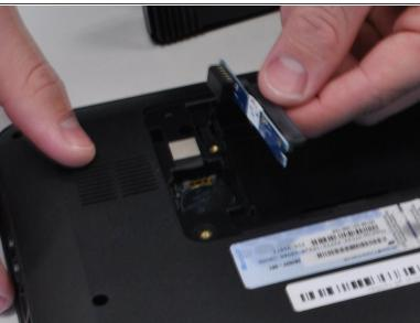
Underneath the computer, unscrew the hard drive connector screw, and pop out the hard drive plug-in.
