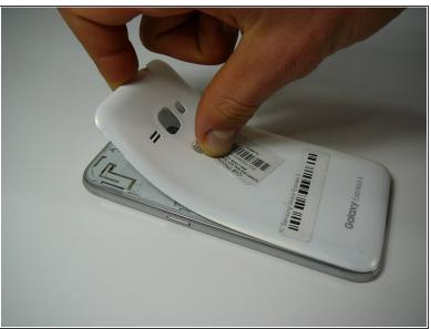
• Locate the indent area highlighted in red and use either your fingernail or a Prying Tool (such as a guitar pick) to separate the back from the body of the phone.
