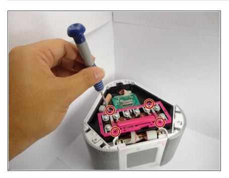
Unscrew the four screws with a Phillips #0 Screwdriver from the pink button sheet.
