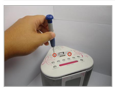
Unscrew the two screws with a Phillips #0 screwdriver on the top side of the device right in front of the eight buttons.
