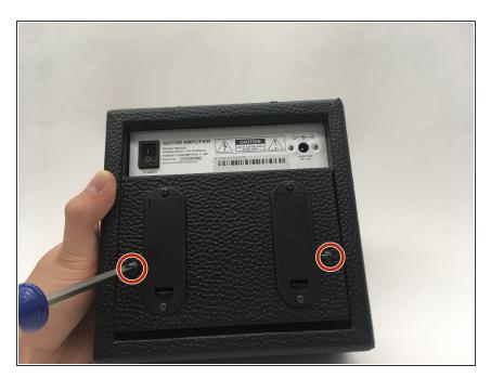
Use a Phillips #0 screwdriver to remove the two 25mm screws that secure back panel to amplifier.
