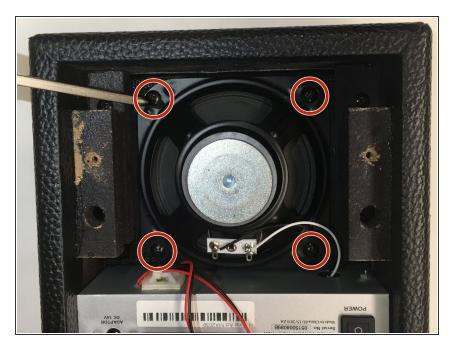
Use a Phillips #0 screwdriver to remove the four 25mm screws that fasten the speaker to the inside of the amplifier.
