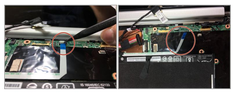
Disconnect the motherboard to powerboard cable from the motherboard using the pointed end of a plastic spudger.
