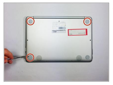
Remove three of the rubber feet on the bottom cover with a plastic or metal spudger.
