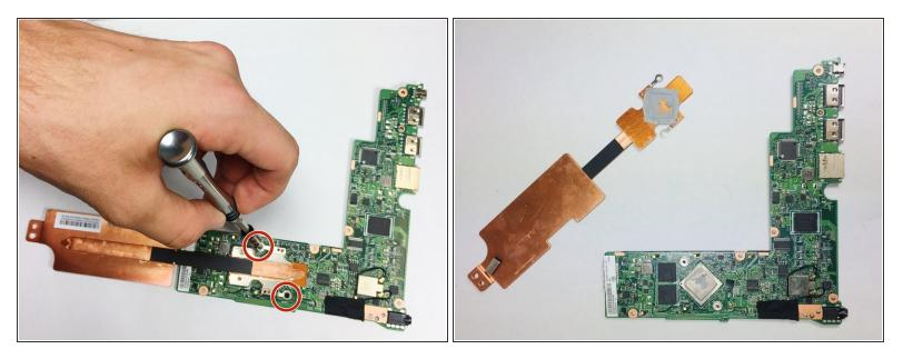
Remove the two 2.7mm heat sink screws with a T5 screwdriver, then remove the heat sink from the motherboard.
