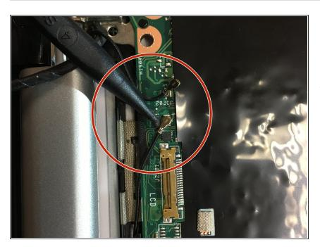
Disconnect the two WiFi antenna cables from the motherboard using the pointed end of a plastic spudger or simply by pulling the cables apart from the motherboard with your fingers.
