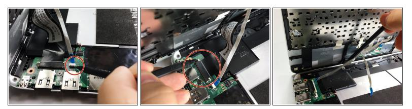
Disconnect the touchpad cable and the keyboard cable on the palm rest assembly from the motherboard using the pointed end of a plastic spudger.
