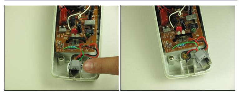
• Slide the phone jack out from the shell by gently lifting up the female phone jack connector.
