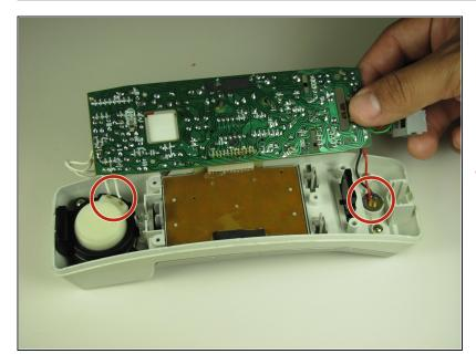
Without removing the motherboard completely, pull up slightly and pivot the motherboard out of the shell.
