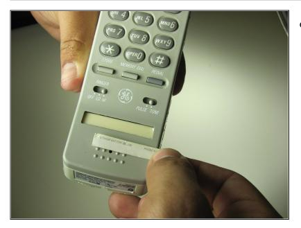
Remove the paper with a plastic opening tool by gently sliding the tool underneath and prying the paper away from the phone.
