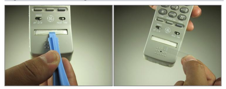
• Remove the plastic cover with a plastic opening tool by gently sliding the tool underneath the plastic and pry the cover off.
