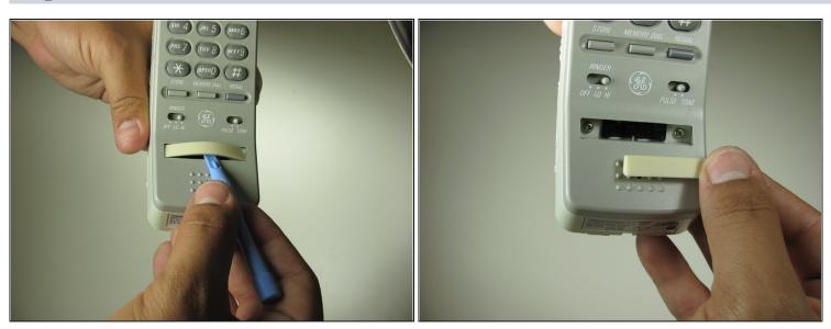
• Remove the rubber stopper with a plastic opening tool by gently sliding the tool underneath and pry away from the phone.
