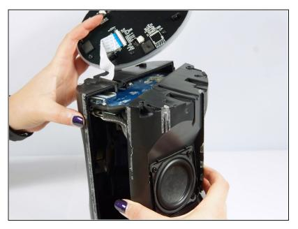
Pry apart the two sides carefully. The halves will not be able to separate completely because of wires and the motherboard.
