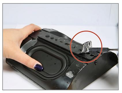
Using the metal spudger, peel the backing off of the back panel of the speaker to reveal 4 screw holes.
