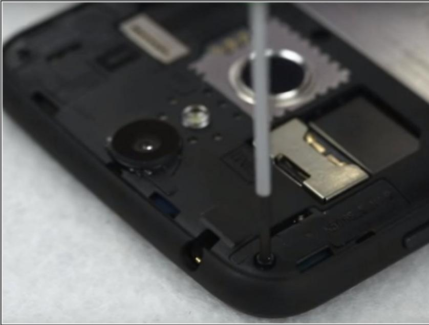
**⚠** Before you proceed, discharge your battery below 25%. A charged lithium-ion battery can catch fire and/or explode if accidentally punctured.
