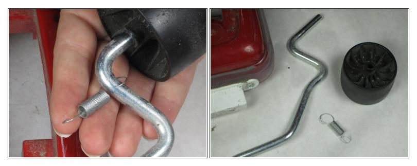
• Remove the wheel from the side with the spring by pulling it off the axel and slide off the spring, as it will be needed for the replacement front wheels.
