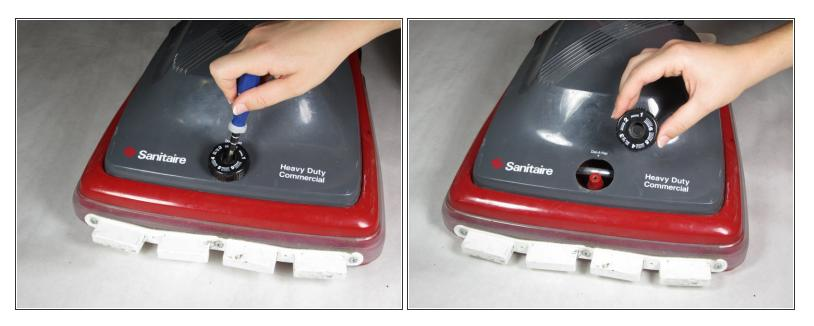
• Stand the vacuum upright, unscrew the single screw located on the center dial using a Torx T20 screwdriver and remove the dial form the vacuum body.
