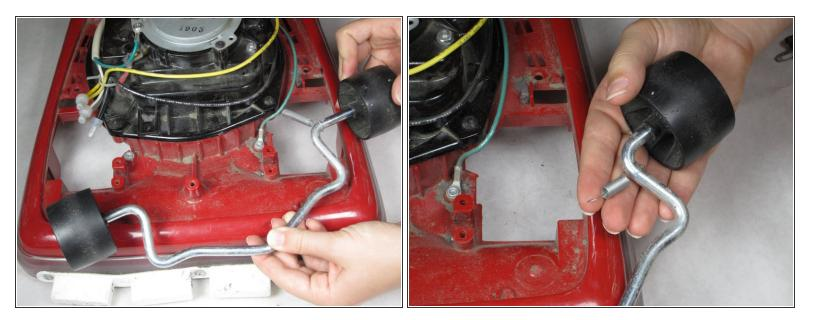
Pull out the silver bar that holds the two wheels to the vacuum body and detach the small spring from the vacuum body.
