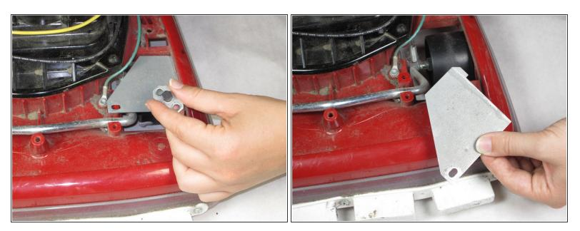
• Remove the small metal plate with the black bolt in the center and the larger gray plate from both sides.
