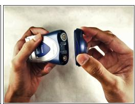
Twist the release cap to expose the batteries.
