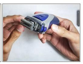
Remove the razor guard by pushing its release buttons and pulling.
