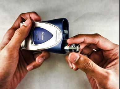
Remove the batteries.
