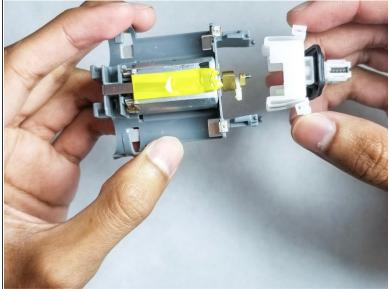
• Detach the white plastic blade base from the tip of the motor by pulling it.
