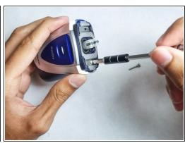
Remove the two 1.9mm Phillips #0 screws from the inner blades.
