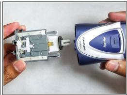
Pull the outer casing with one hand while holding the inner battery casing with the other hand.
