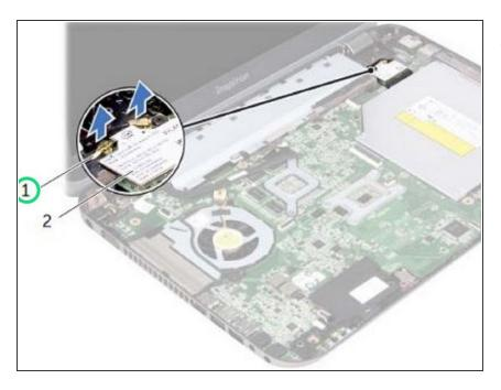
Connect the antenna cables to the connectors on the Mini-Card.
