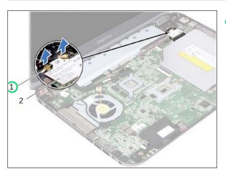
Disconnect the antenna cables from the connectors on the Mini-Card.
