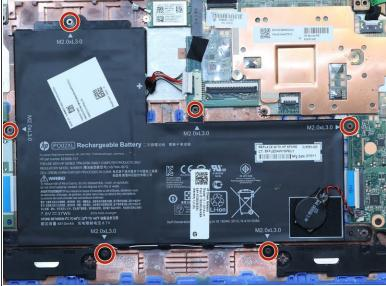
• Use a Phillips #00 screwdriver to remove six 5 millimeter screws from the battery.
