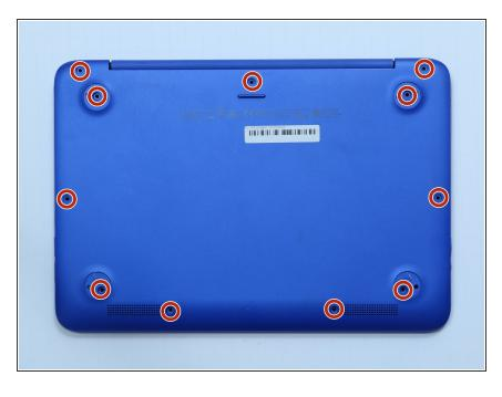
Remove the eleven 5 millimeter housing screws from the bottom of the computer using a #00 Phillips head screwdriver.
