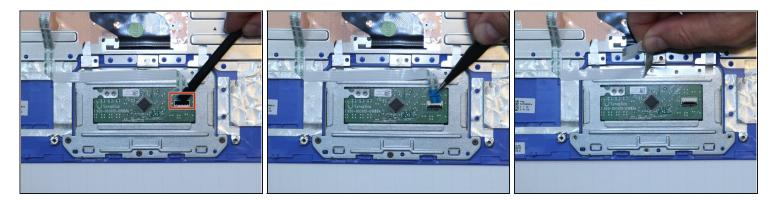
• Use a plastic spudger to remove the black, plastic tab holding down the ZIF connector.
