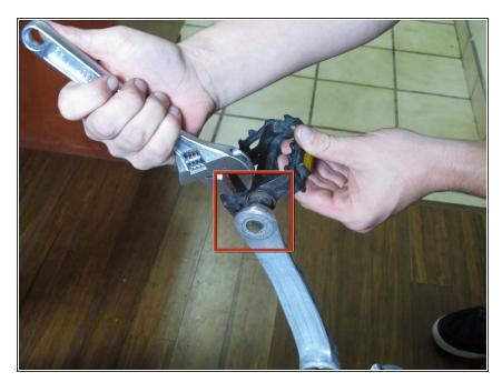
Use an 8" adjustable crescent wrench to fit it into the base of the pedal.
