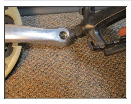
Turn the wrench continuously until the pedal detaches from the crank arm.
