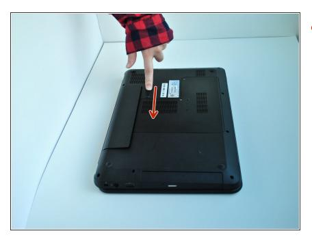
Slide the switch under the battery compartment to release the battery.
