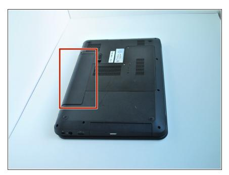
Flip the computer so that the bottom side is facing up, and locate the battery above the screen hinges.
