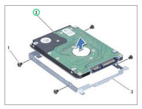
Lift the hard drive out of the hard drive bracket.
