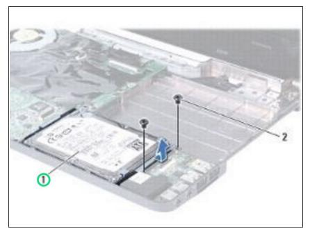
Slide the hard drive assembly to the right to disconnect it from the connector on the system board, then lift the hard drive assembly out of the computer base.
