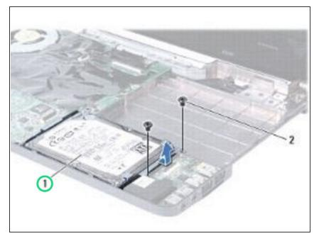
Place the hard drive assembly in the computer base and push to connect the hard drive assembly to the connector on the system board.
