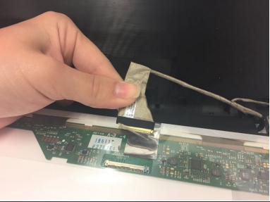
On the back of screen, lift up the plastic film and screen connector. Pop out the connector, and gently remove the screen. To reassemble your device, follow these instructions in reverse order.
