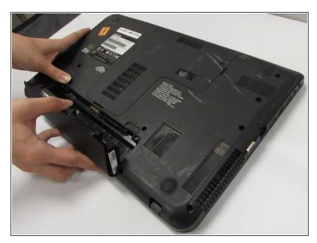
Lift and remove the battery from the device.
