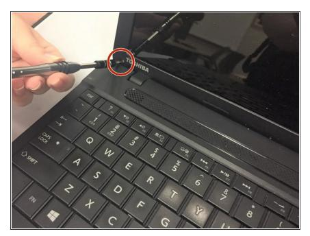
Use the Phillips #1 screwdriver to unscrew the two screws in the lower corners of the screen.
