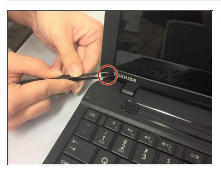
Use tweezers to remove the screw covers in the lower corners of the screen.
