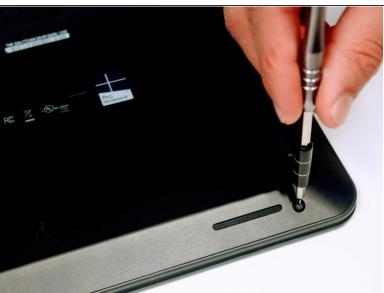
Remove the 8 screws holding down the back panel using the Phillips screw driver #000.
