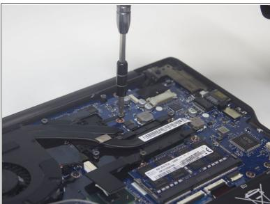
Remove the 9 wafer-head screws, size M2x4mm, using the Phillips screwdriver #000.
