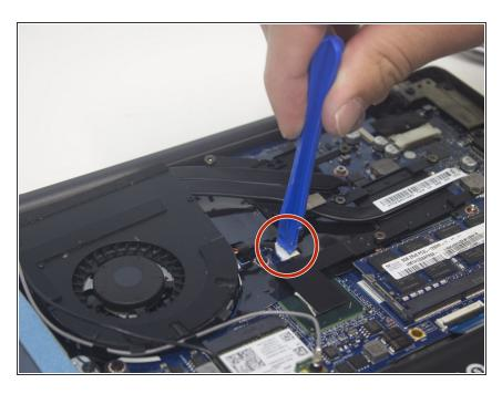
Remove the fan's cable using the plastic opening tool.
