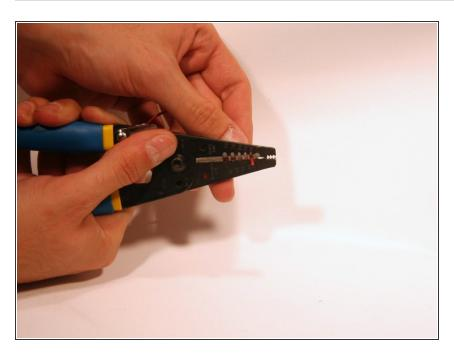
Place the wire stripper about a 1/4" from the end of the wire and squeeze down.
