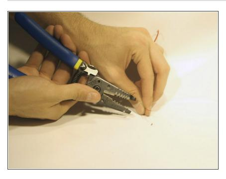
While squeezing, pull the stripper along the end of the wire. This should expose some of the wire by removing its insulation.
