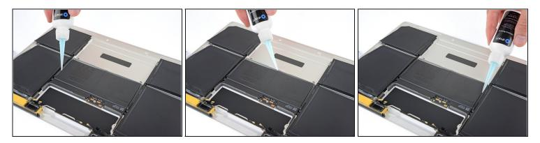
• Lay the lower case assembly down flat, and apply adhesive remover to the two middle battery cells—at each side, and along the front edge (opposite the logic board area).
