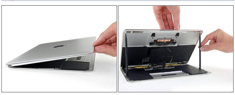
Lift the upper case and display together from the front edge and raise it to about a 45° angle.
