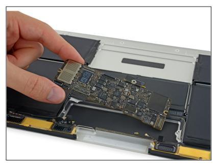
• Remove the logic board.
