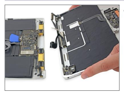
• Separate the upper case assembly from the lower case assembly.
