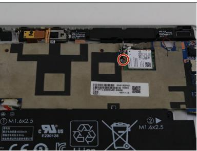
Use a Phillips #0 screwdriver to remove the screw from the left hand side of the board.
