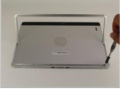
• Use a T5 driver to remove the six screws on the back of the tablet.
