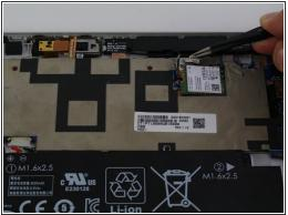
Remove the two black wires that are connected to the board with a pair of tweezers.
