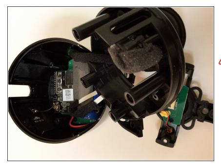
After removing all of the screws from the plastic cover, remove it by pulling up and out.
