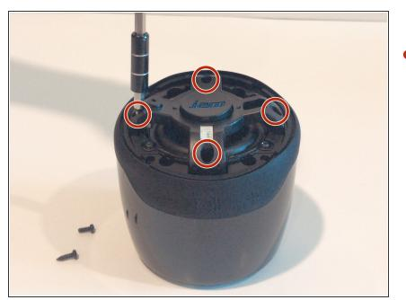
Remove the four 7mm Phillips screws from the plastic cover.
