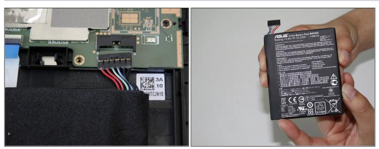
• Remove the battery from the device.
