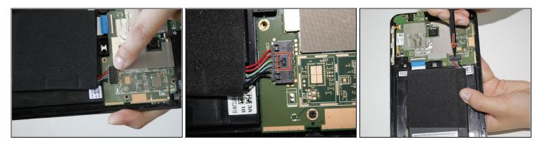
• Using the spudger, gently press on the black button on the plug port to release the battery from the plug.
