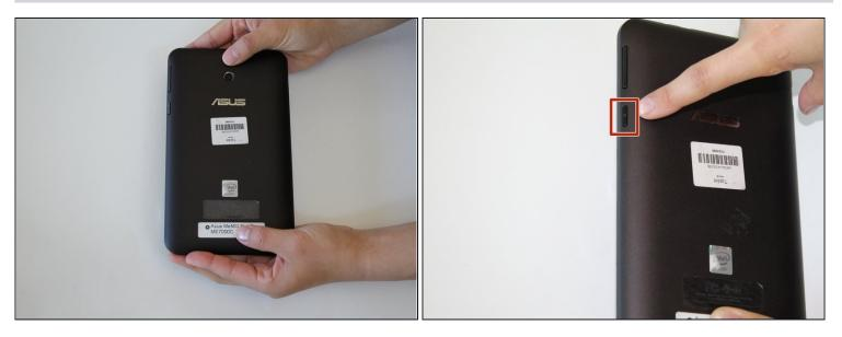
• Flip over the tablet so the back cover is facing you. Hold the second button on the left below the volume buttons down until it powers off.
