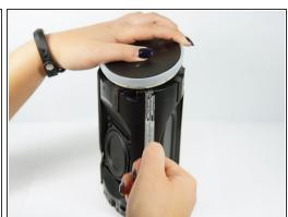
Peel off all rubber strips along sides, middle front and middle back of the device.
