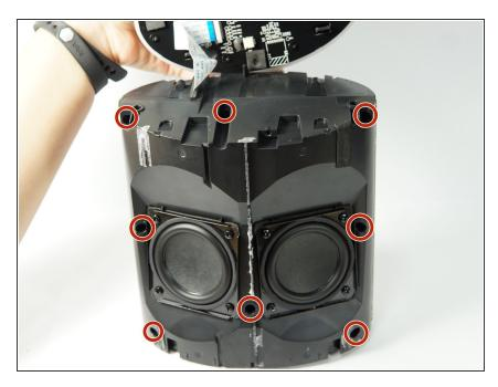
Remove the eight 6 mm screws using the Phillips #2 screwdriver.
