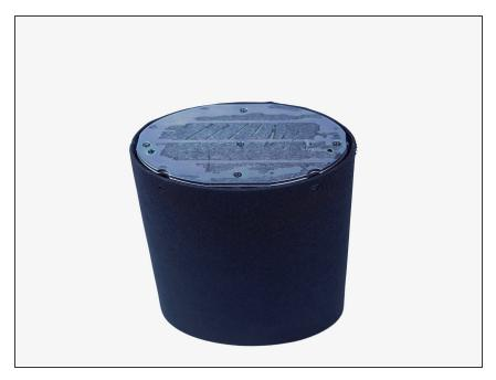
Scrape most of the glue away to reveal the five flathead screws - four around the outside, and one in the middle.
