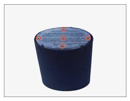
Remove the five 6 mm screws with a Phillips #2 screwdriver.
