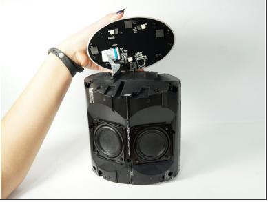
Carefully remove the top panel, light ring, button panel, and the corresponding board.
