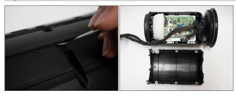
• Pry the two halves of the body open using a metal spudger.
