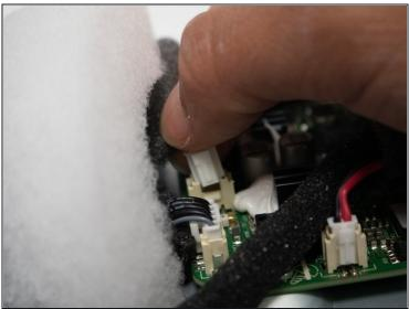
• Disconnect the plug in the device.
