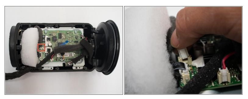
Disconnect the plug in the device.
