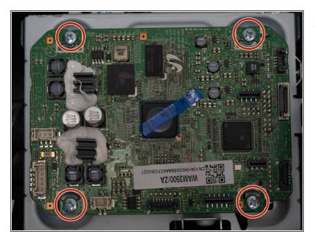
• Remove the four 12mm long screws with the Phillips #1 screwdriver .
