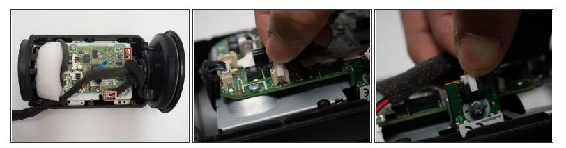
• Remove the plugs located topmost right and closest to the bottom in picture.
