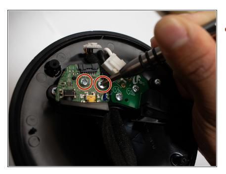
Remove the two 10mm long screws from the board utilizing the Phillips #1 screwdriver.
