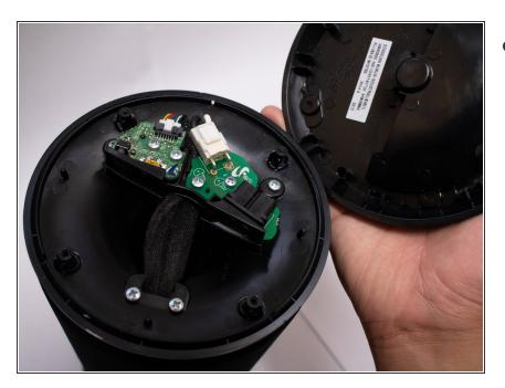
Remove the bottom shell from the speaker.
