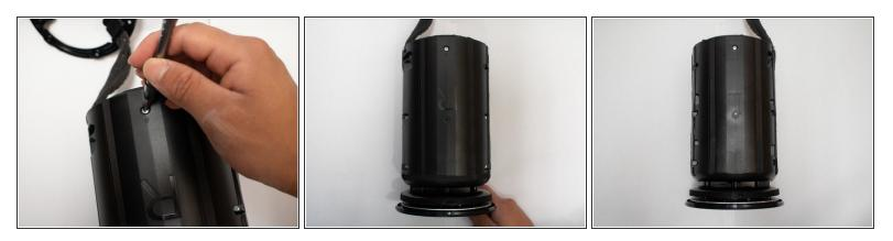
• Remove the eight 12mm long screws around the body with the Phillips #1 screwdriver.
