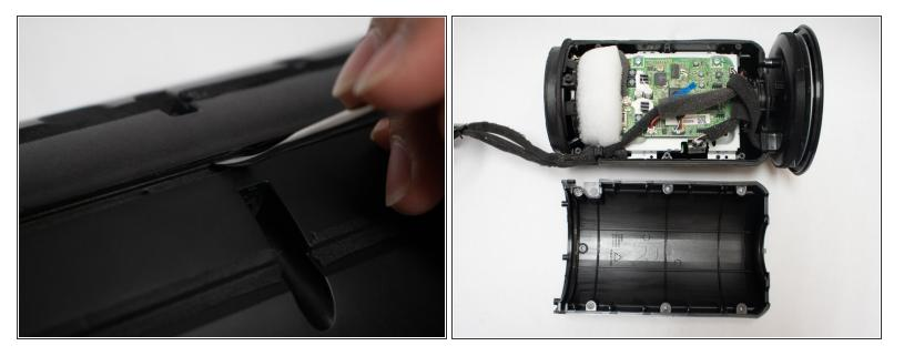
• Pry the two halves of the body open using a metal spudger.
