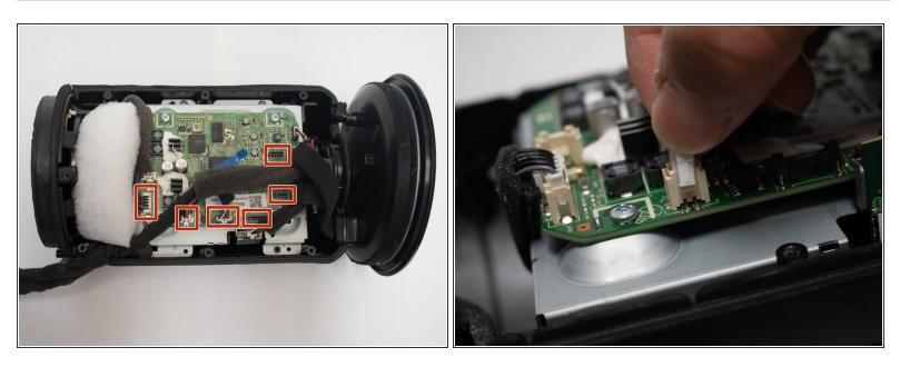
Disconnect the six plugs on the motherboard.
