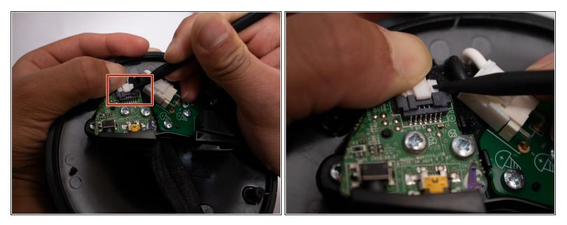
Remove the connector from the board by pressing down on the center tab while nudging the connector away with a spudger.
