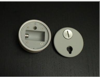
The back of the Sensor has a simple screw, which gives us access to the battery
