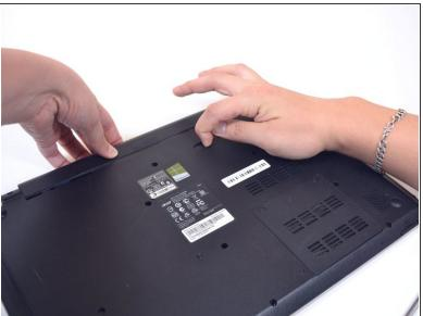
Slide the locking latch to the right and hold while pulling the battery out with your other hand.
