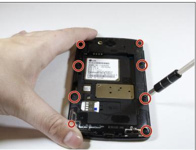
Use the phillips #000 Screwdriver to unscrew eight 4mm screws.
