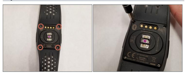
• Remove the four 6.7mm JIS #00 screws from the back cover.
