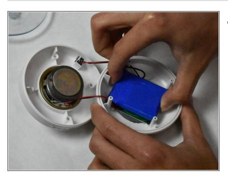
Hold the base and pull up on the battery.
