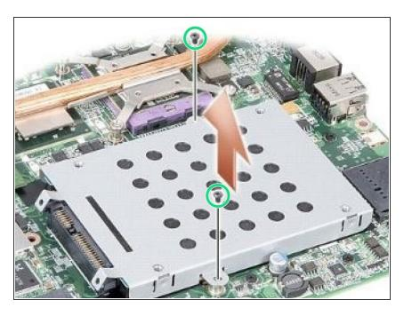
Replace the two screws securing the hard drive assembly to the system board.
