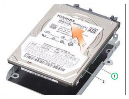
Press down on the hard drive at the non-connector end slot to remove the hard drive off the hard drive cage.
