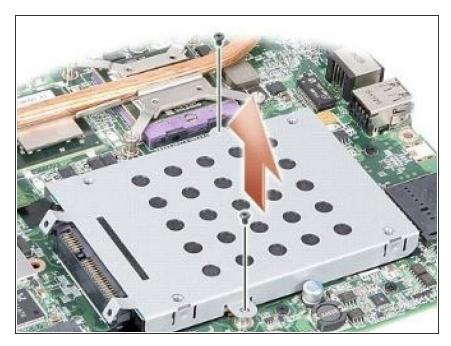
Push down the hard drive assembly in place by aligning the hard drive connector with the system board connector.
