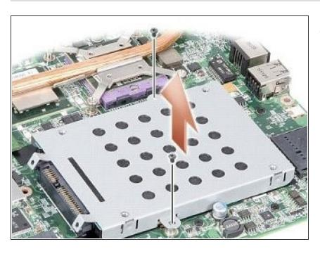
Holding the connector end of the hard drive assembly, pull the hard drive assembly from the system board connector.
